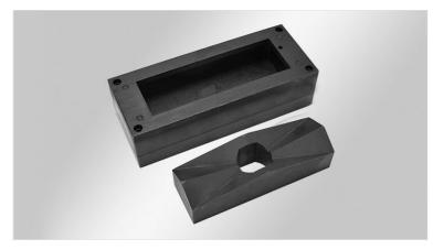
Rectangular and square punches and dies make it easy to punch holes into stainless steel (V2A versions), mild steel, aluminium or plastics with a max. sheet thickness of 2 mm. Available for cut-outs sizes of 10-, 16-, and 24- multi-pin heavy industrial connectors and also for numerous special cut-outs. Therefore, the punches are suitable for most icotek cable entry systems. Centre punches are integrated in the die for exact drilling of mounting holes.
